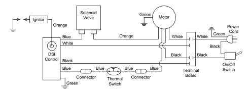
Figure 11 - Wiring Diagram
